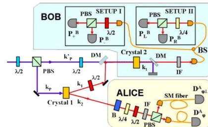
FIG. 1 (color online). Configuration of the quantum injected optical parametric amplifier. The polarization entangled photon couple is generated by crystal 1, while crystal 2 realizes the optical parametric amplifier (OPA) action.
