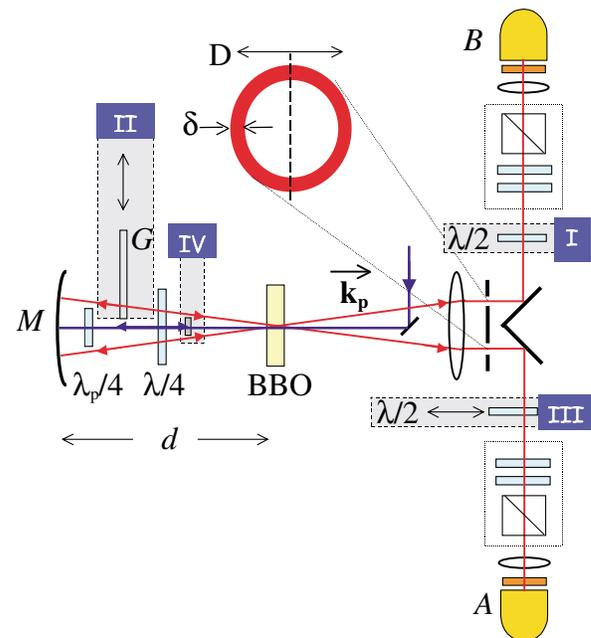
FIG. 1 (color online). Layout of the high brilliance source of polarization entanglement. The two dashed boxes located before detectors  $A$  and  $B$  represent the system for tomographic reconstruction of the produced states.
