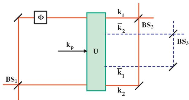
FIG. 1 (color online). Schematic diagram of the nonlinear Mach-Zehnder interferometer (MZ-IF) terminated at two different correlated frequencies.
