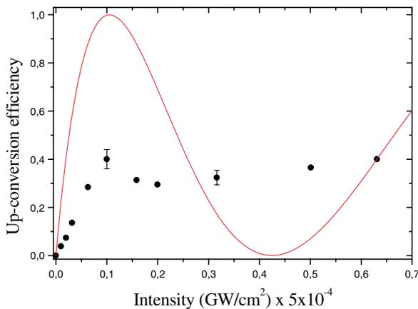
FIG. 3 (color online). Up-conversion quantum efficiency QE as a function of the laser pump intensity  $I_p$ ; theoretical (continuous line) and experimental results.
