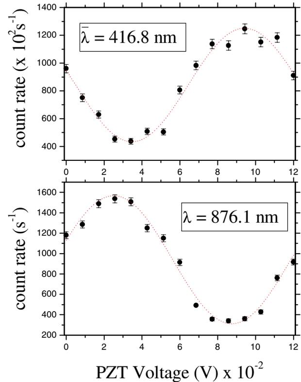
FIG. 4 (color online). Single photon interference fringes obtained within the same experiment at the different correlated wavelengths  $\lambda$  and  $\bar{\lambda} = (\lambda^{-1} + \lambda_p^{-1})^{-1}$ . The phase period of the fringing patterns is in agreement with the figure of merit (0.7 nm/V) of the piezoelectrical transducer activating the mirror M.
