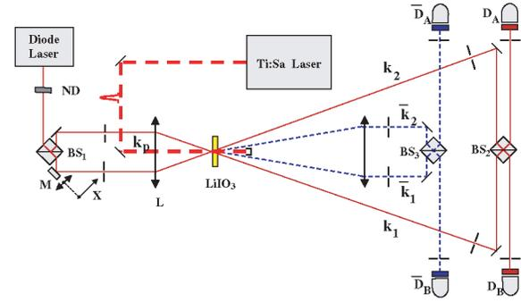
FIG. 2 (color online). Layout of the single-particle MZ-IF experiment.
