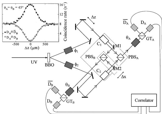
FIG. 1. The experimental arrangement. The dotted lines show the invar table and slide used to vary  $\Delta x$ . The inset shows a typical scan over  $\Delta z$  showing visibility of about 92%.
