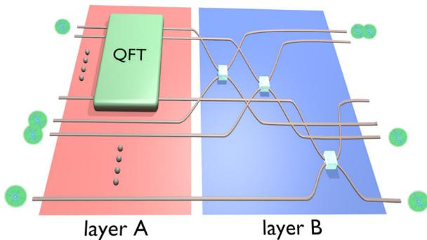
FIG. 1. Family of interferometers capable of witnessing genuine  $n$ -photon indistinguishability. QFT is the quantum Fourier transform acting on  $(n - 1)$  modes. Each output of the QFT is connected to a 50/50 beam splitter. As discussed in the main text, no mixture of states with less than  $n$  indistinguishable photons can result in a probability of bunching  $p_b > [(2n - 3)/(2n - 2)]$ .
