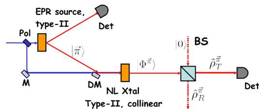
FIG. 1 (color online). Amplified states of the collinear optical parametric amplifier injected by a single-photon qubit generated in a type-II EPR source. Beam-splitter (BS) loss model for the amplified macroscopic states generated by the collinear QI-OPA.
