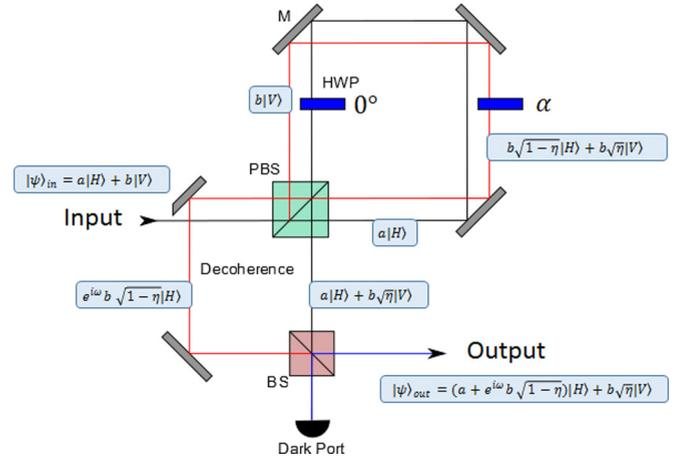
FIG. 5. Scheme of the experimental implementation of the AD map  $\mathcal{A}_\eta$  via a DIF loop. In this picture path **a**, associated with the  $|H\rangle$  polarization component, is indicated in black, while path **b**, associated with the  $|V\rangle$  component, is in red. The blue elements represent HPW elements.
