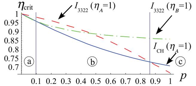
FIG. 5. (Color online) Critical detection efficiencies in the completely asymmetric case for the CH and the Collins-Gisin inequalities.  $I_{3322}$  with  $\eta_A = 1$  (dashed line) and with  $\eta_B = 1$  (dash-dotted line); CH (solid line). Labels (a), (b), and (c) identify the three ranges where different inequalities lead to the lower efficiency threshold.
