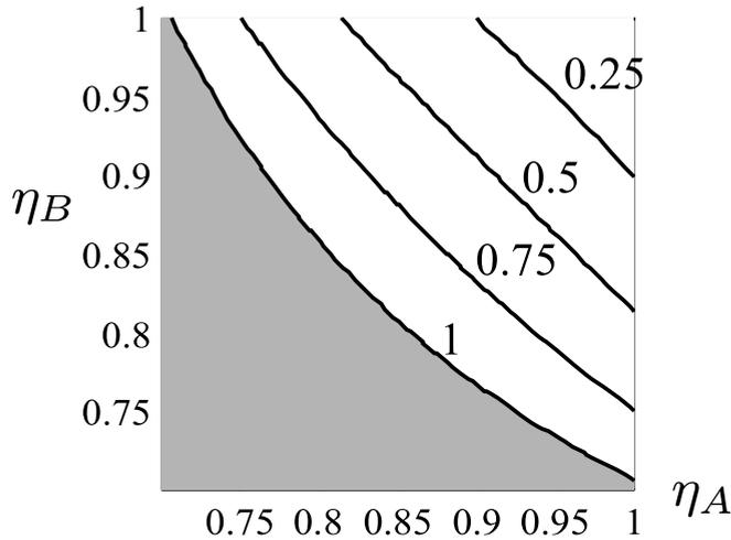
FIG. 4. Allowed values of  $\eta_A$  and  $\eta_B$  for a loophole-free Bell test for different values of  $p$  (1,0.75,0.5,0.25). For each value of  $p$  the allowed zone is in the upper-right part of the corresponding curve.
