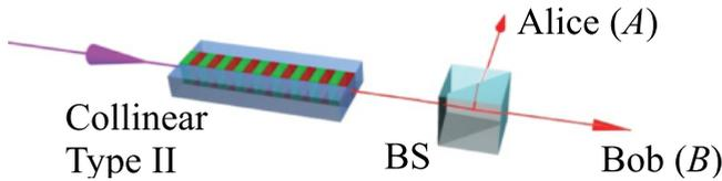
FIG. 1. (Color online) Collinear source of two photon states. The two particles are produced by type II phase matching and randomly broadcast to two observers  $A$  and  $B$  via a beam splitter (BS).
