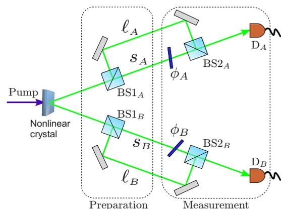
FIG. 1. (Color online) Scheme of Franson's interferometer. The long and short arms are labeled as  $\ell$  and  $s$ , respectively. The thin glasses ( $\phi_A$ ,  $\phi_B$ ) can be used to change the phase in the measurement.
