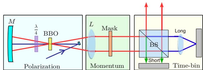
FIG. 8. (Color online) Scheme for the generation of two-photon polarization and momentum and time-bin entangled states.
