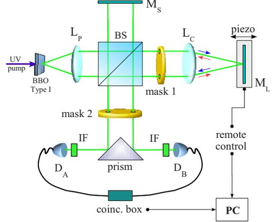
FIG. 2. (Color online) Michelson interferometric scheme used to generate time-bin entanglement.
