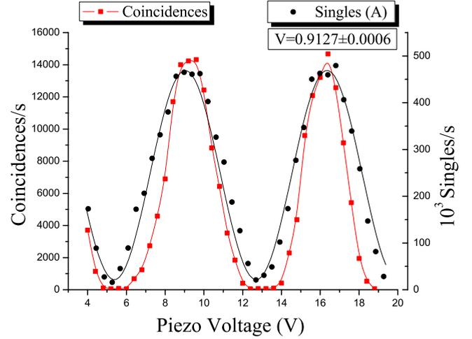
FIG. 3. (Color online) Single (right) and coincidence (left) counts measured by our apparatus in the presence of single photon interference. The high visibility of the single count oscillation is used to test the correct position of the lens  $L_P$ . Coincidence counts also oscillate in agreement with Eq. (4).
