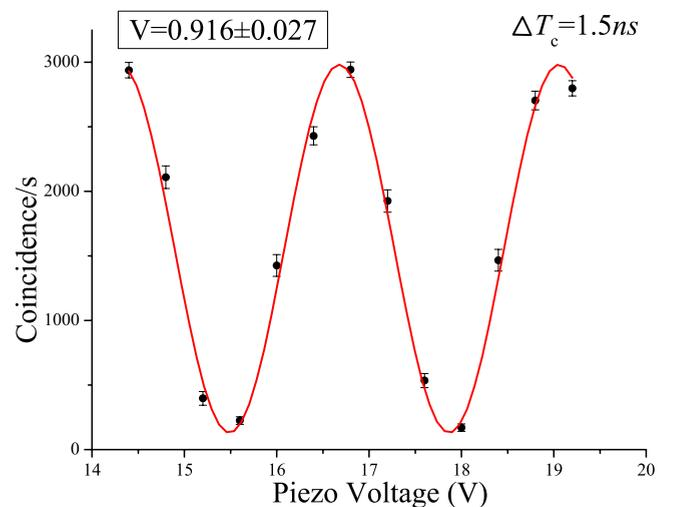
FIG. 4. (Color online) Coincidence counts after accidental coincidence subtraction with  $\Delta T_c=1.5$  ns in the case of time-bin entanglement. Error bars are calculated by considering both the Poissonian statistic and the uncertainty of the voltage applied to the piezo transducer.
