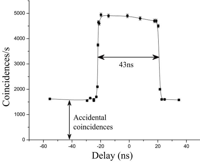
FIG. 5. Measurement of a coincidence window  $\Delta T_c=21.5$  ns. Fixing the arrival time of the first photon, we measured the coincidences by varying the arrival time delay of the second photon. The baseline ( $\sim 1600$  coinc/s) corresponds to the accidental coincidence contribution. This value is in agreement with that obtained by Eq. (13).
