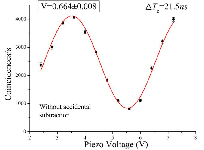
FIG. 6. (Color online) Raw coincidence counts (without accidental coincidence subtraction) with coincidence window  $\Delta T_c=21.5$  ns.
