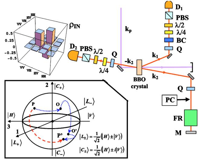
FIG. 1. Experimental setup adopted for the characterization of the FRM reflection process. Inset: Representation of the FRM action on the Poincaré sphere. The tomographic reconstruction of the input singlet state  $\rho_{k_1,-k_2}^{in}$  is reported. It was obtained by direct measurements taken on the mode  $\mathbf{k}_2$ , i.e., by replacing FRM with the whole measurement apparatus terminated by  $D_2$ .
